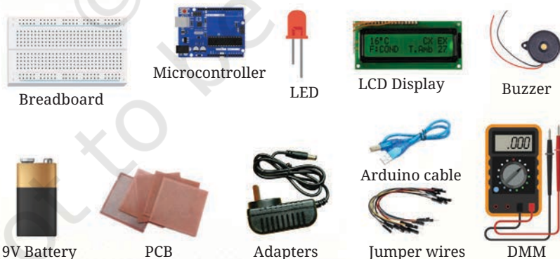
Figure 4.3: Electrical and electronic components
