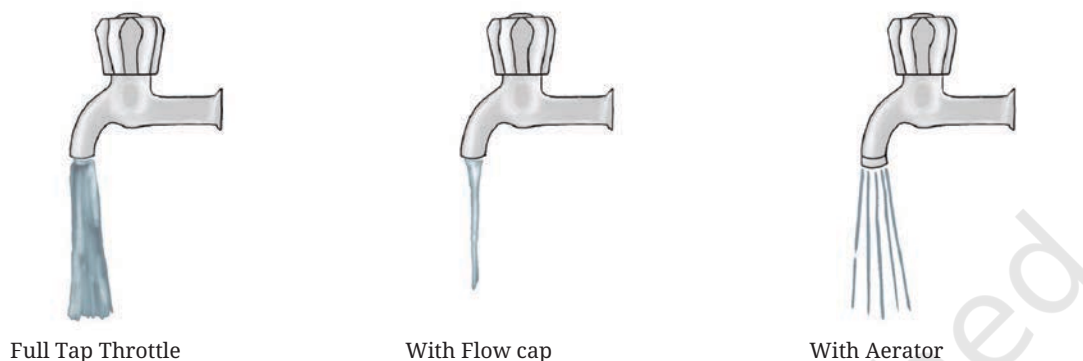
Figure 5.10: Comparison of water flow with and without flow cap and aerator
